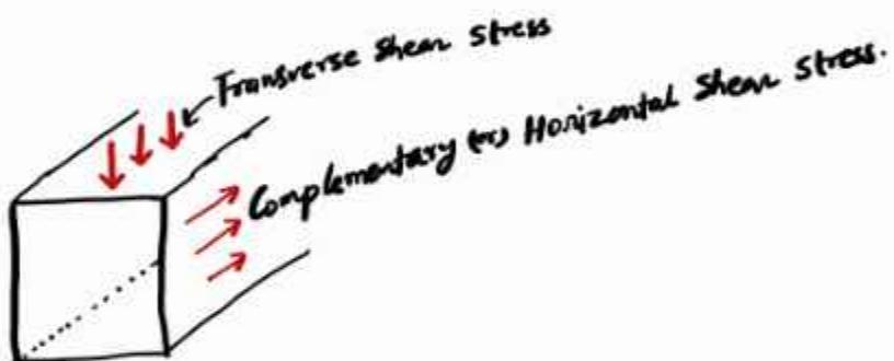
The applied shearing force will be distributed as a shearing stress across transverse sections of the beam. At each point on the section the transverse shearing stress will produce a complementary 'horizontal' shearing stress.
